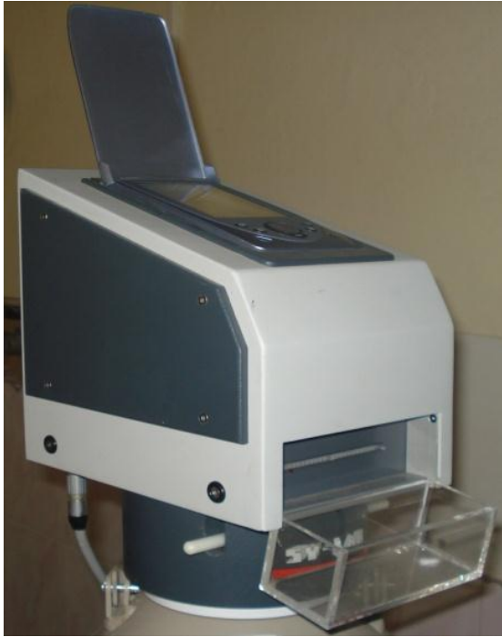
Fig-3: Bio-freezer with inbuilt seeding rod
